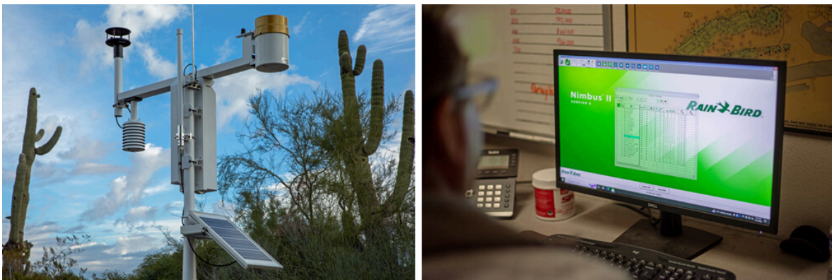
Weather stations on the course at Grayhawk (left) relay data to software (right) that Ernie Pock uses to determine how much water is needed.
